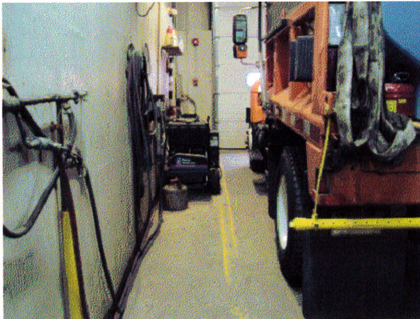
Figure 19: Equipment stored in the side access aisle further limits access to vehicles in the wash bay.
