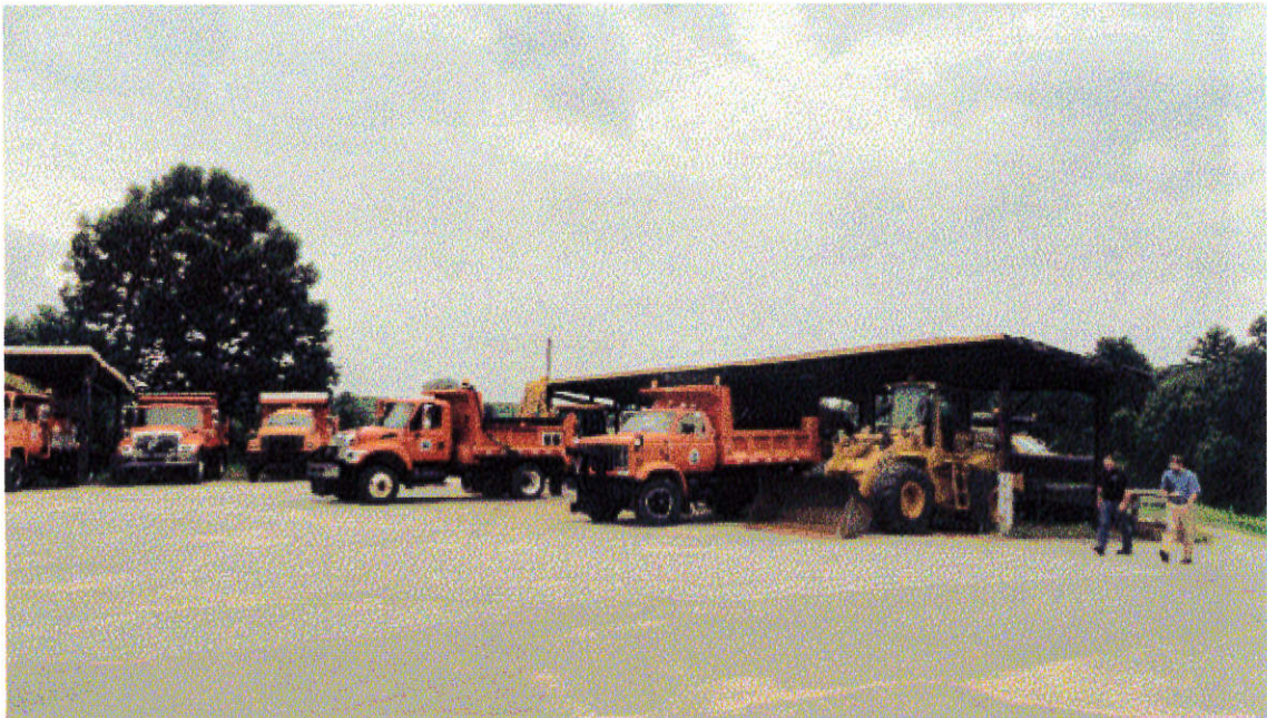
Figure 5: Two shed roof canopy structures provide some shelter for construction equipment. The lack of enclosed garage space means that half of the town's fleet is exposed to the weather.
