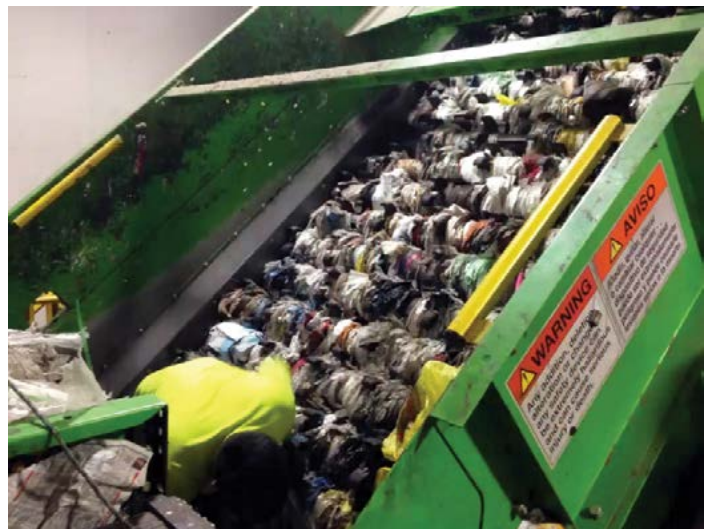
Employee (yellow shirt) removes plastic film from sorting machine.
