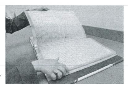
This construction allows for a flat book block and reinforces the binding edge for added strength and years of service. Available in custom sizes, the Pocket dimensions will match the 'book block' dimensions with a 1½" or 1¼" binding margin.
