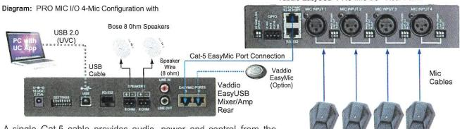
A single Cat-5 cable provides audio, power and control from the EasyUSB Mixer/Amp to the PRO MIC I/O. This configuration can be used in conjunction with an EasyMic Table MicPOD providing maximum flexibility in design. Up to two (2) PRO MIC I/O Interfaces can be connected to a single EasyUSB Mixer/Amp for a complete 8-Microphone USB Audio Conferencing solution.
