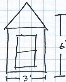
Gabled Dormer typically 2:1 (H:W)
